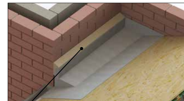
47.5mm packed off timber has been used to pack off the box gutter to line up with the standard gutter.
