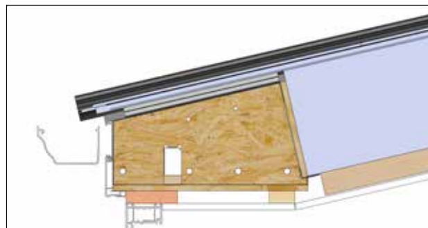
This image is showing the plaster line at 12.5° to 15° using 100 x 25mm timber packer (not supplied)
